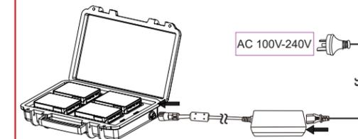
\* Rotate the DC plug counterclockwise to detach the power adapter.
